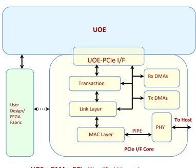
UOE + DMA + PCIe (Simplified Diagram)
